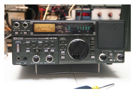
Checking all of the modes and functions, I notice a significant pitch change when shifting from LSB to USB so there are likely more alignment issues, possibly with the BFO or the pass band tuning circuits, which need to be dealt with. I'll get to those when I have another day with no other pressing projects.
