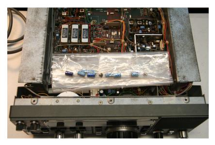
With covers removed, I take a quick look for burnt components, missing parts, disconnected leads, bulging electrolytic capacitors etc. Finding none, I suspect there is a glimmer of hope this Receiver is repairable. I also note this Receiver has an optional InRad SSB XTAL filter in 455 KHz IF section!
